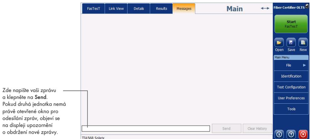
The screenshot shows the 'Messages' window of the Fiber Certifier OLTS software. The interface is divided into several sections:
