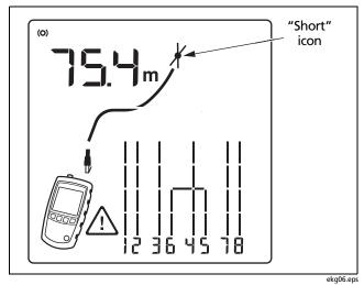
Figure 7. Short on Twisted Pair Cabling
