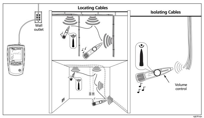
Figure 25. Using the Toner in IntelliTone Mode
