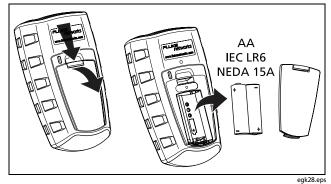
Figure 28. Replacing the Tester's Batteries
