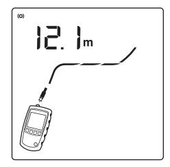
Figure 20. Open on Coaxial Cabling
