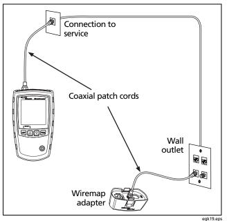
Figure 18. Connecting to Coaxial Cabling
