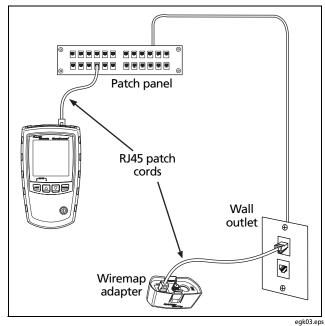
Figure 5. Connecting to Twisted Pair Network Cabling
