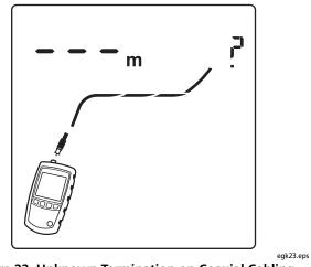
Figure 22. Unknown Termination on Coaxial Cabling
