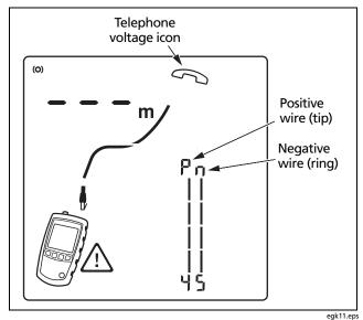
Figure 11. Telephone Voltages Detected
