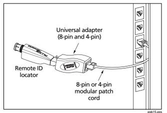
Figure 4. Connecting a Remote ID Locator in a Confined Area or to an RJ11 Jack
