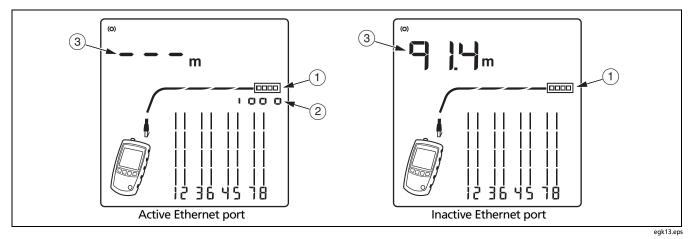
Figure 13. Ethernet Port Detected
