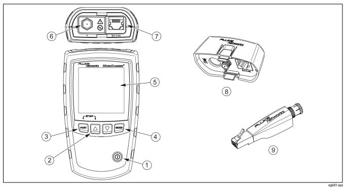
Figure 2. MicroScanner<sup>2</sup> Features
