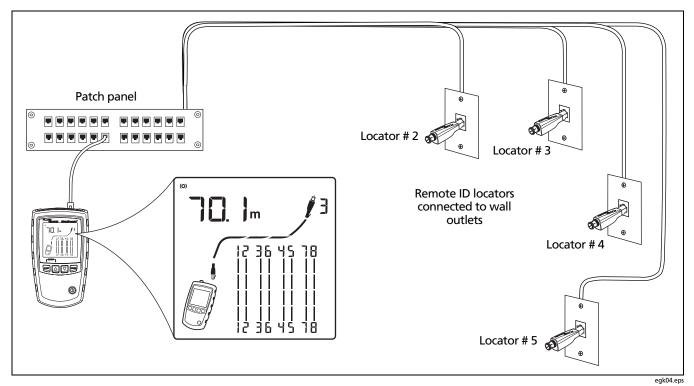
Figure 15. Using Multiple Remote ID Locators
