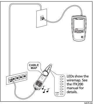
Figure 27. Using the Toner with the IP200 IntelliTone Cable Map Function
